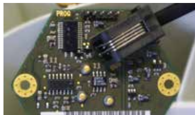
Solvents detection sensor
