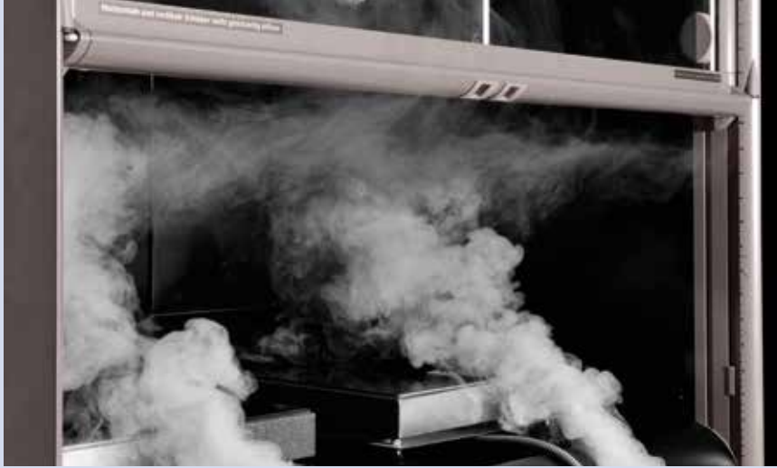
Standard fume cupboard with heating source
