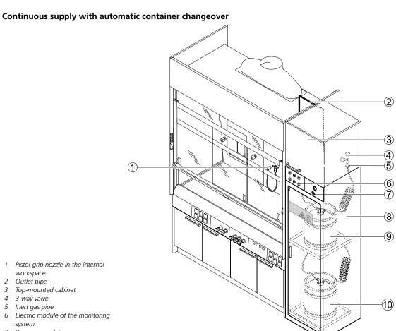
Supply system for flammable liquids
