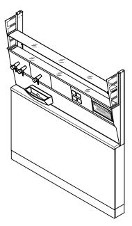
Service spine for wall bench with underbench units on plinth and media supply from above, working height 900 mm
