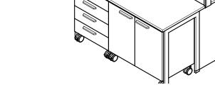
Bench-mounted service duct with overbench cabinets, pillar extension and underbench units on plinth
