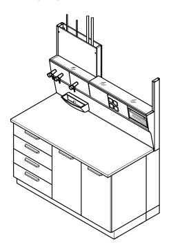
Service spine for wall bench with C-frame, underbench units on castors and overbench cabinet, working height 750 mm
